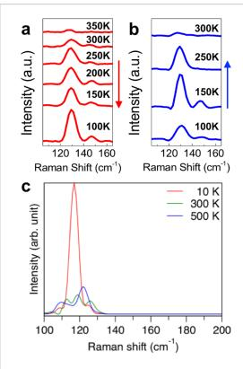
**Figure 5.** (a) Temperature dependent Raman spectra of PVD-grown tellurene flake (on as-grown substrate) while heating (100 K–350 K) and (b) cooling (RT—100 K) showing evolution of the  $A_1$  and  $E_{\rm TO}$  mode intensities, widths, and positions. (c) Simulated Raman spectra of a tellurene film at 10 K, 300 K and 500 K show a depression of Raman intensity for the  $A_1$  mode.
