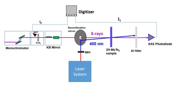
FIG. 1. Schematic of the experimental setup at PAL-XFEL (not to scale). The incident x-ray intensity ( $I_0$ ) of each pulse is measured using the ejected photoelectrons from an  $Si_3N_4$  membrane detected with an MCP detector. The transmitted x-ray intensity through the sample ( $I_1$ ) is measured with a photodiode.
