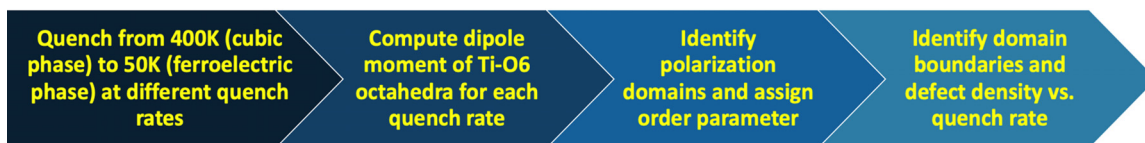
FIG. 3. Workflow for quenching schedule and identifying defects in BTO.
