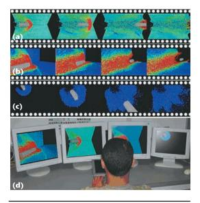
Figure 10. A scientist investigates the hypervelocity impact damage caused by a projectile using the multimodal, mulitdisplay visualization system. The top three images show (a) the pressure distribution, (b) temperature, and (c) coordination number in the MD system across time. The fourth image (d) shows a scientist simultaneously viewing the different modalities from different viewpoints.
