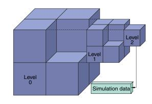
Figure 2. A three-level octree implementation. Each octree node contains the coordinate bounds of the corresponding subspace. A terminal node at level 2 points to a structure that stores data associated with atoms in the region defined by the terminal node.
