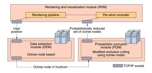
Figure 7. Parallel and distributed implementation of Atomsviewer. By delegating data-reduction functions to the two nongraphic modules (DEM and POM) and dedicating the graphics server (RVM) to rendering, we significantly increase the frame rate.
