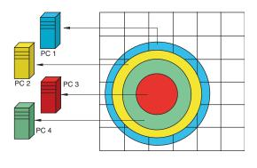
Figure 8. The parallel implementation of the octree-based view frustum culling. The concentric shells, each of equal volume, are distributed over a PC cluster to perform a coarse extraction of octree regions.
