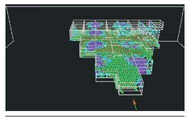
Figure 3. The octree data structure overlain on the atomistic data. The figure shows only the atoms that are selected for subsequent rendering.
