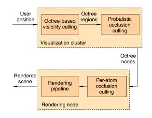
Figure 1. Overview of the Atomsviewer visualization system. To prevent bottlenecking caused by polygon rendering, the system processes only those data that the viewer will see.
