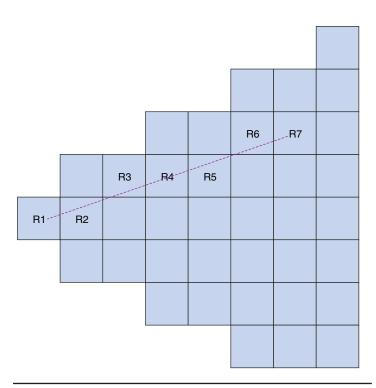
Figure 4. Probabilistic occlusion culling. The viewer is in region R1. To calculate the visibility of region R7, for example, we trace a line from R7 to R1 and calculate the visibility using the visibility of the regions along this line. The visibility of R7 is therefore a function of the visibility of R6 and the distance of R7 from R1.
