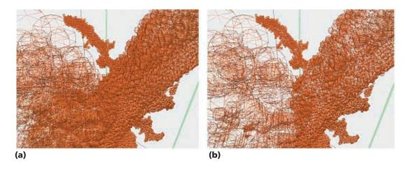
Figure 6. A wireframe rendering of a scene (a) without occlusion for rendering and (b) with occlusion for rendering. Figure 6a is rendered at 0.94 frames per second and includes 90,000 atoms. Figure 6b is rendered at 3.22fps and includes only 4,500 atoms.
