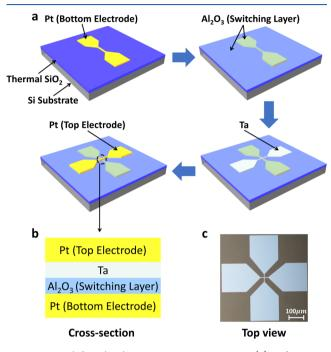
Figure 1.  $Pt/Al_2O_3/Ta/Pt$  cross-point memristor. (a) Fabrication process. (b) Schematic of the  $Pt/Al_2O_3/Ta/Pt$  cross-point memristor. (c) Optical microscope image of the fabricated  $Pt/Al_2O_3/Ta/Pt$  cross-point memristor.
