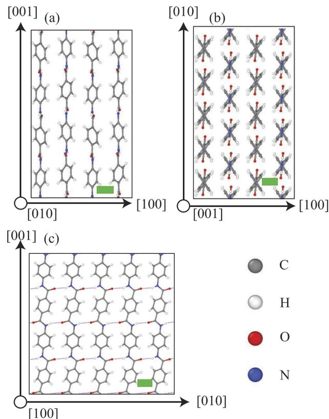
**FIG. 1.** Structure of the PPTA crystal with views from (a) [010], (b) [001], and (c) [100] directions. Scale bar dimension in (a)–(c) is 2.5 Å. Hydrogen bonds are indicated by dotted lines. (a)–(c) Produced with OVITO version 5.3.3.
