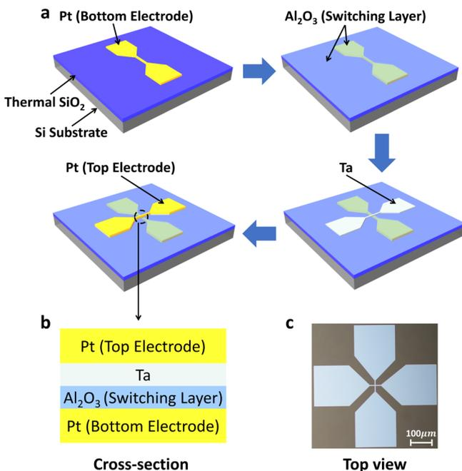
**Figure 1.** Pt/Al<sub>2</sub>O<sub>3</sub>/Ta/Pt cross-point memristor. (a) Fabrication process. (b) Schematic of the Pt/Al<sub>2</sub>O<sub>3</sub>/Ta/Pt cross-point memristor. (c) Optical microscope image of the fabricated Pt/Al<sub>2</sub>O<sub>3</sub>/Ta/Pt cross-point memristor.
